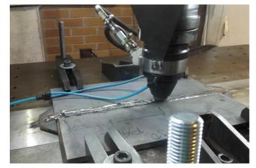
FSP preliminary trials performed in AIMEN on homogeneous sample S690 material
